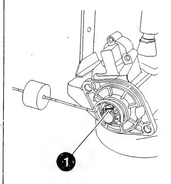
Checking armature braking torque
